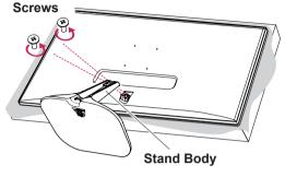
1 Turn the screw to the left. 2 Pull out the Stand Base.
